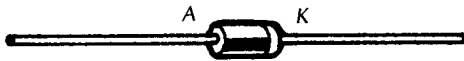
A typical diode with a band at one end to indicate the cathode (K).
